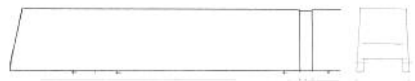
My working sketch for cutting and assembling the body panels from 40 thou clear plastic sheet.
