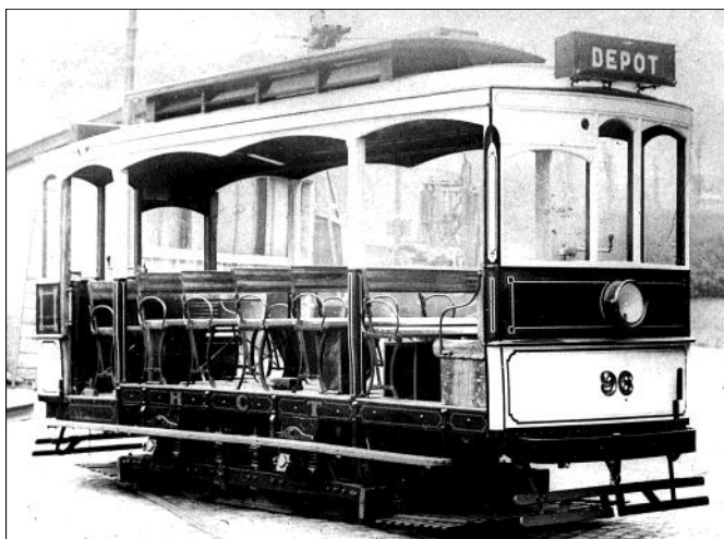
Above: Started by BEC but finished by Brush at the end of 1904 were Halifax cars 95 and 96. Initially they were two-window versions similar to those at Gravesend, but 96 was converted to a crossbench car in 1906 as seen here.
